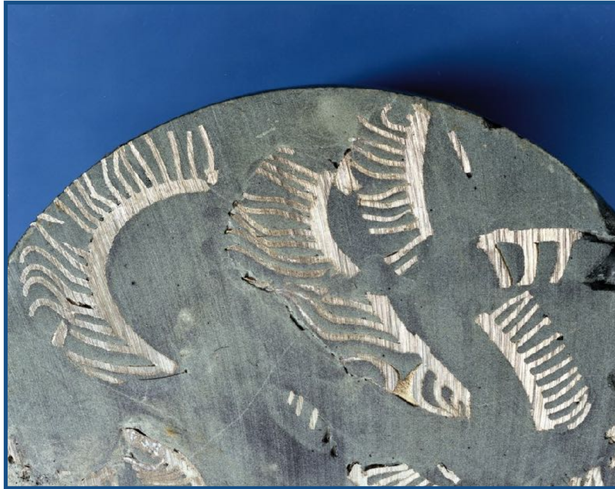
ILW Cross Section, Cladding & Grout
