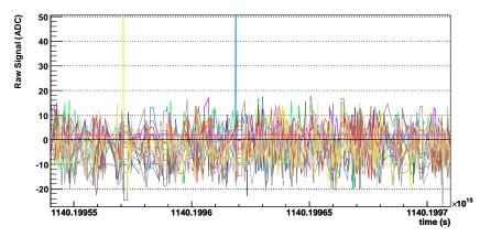
one readout chip, ADC minus mean of first 20 events.
